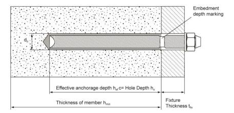
Anchor application in hollow/perforated masonry with nylon sleeve (brick  $n^\circ 2$  according to Annex B9)
