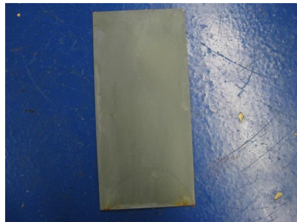
Picture 16 Zinc 240 30-50µm after 2000 h condensation water test
